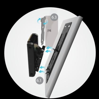
6.1 Hang the screen on the bottom hooks. 6.2 Rotate the screen up to hook the top hooks. 6.3 Tighten the security screw. (Use a screw removed from the screen plate in step 1.)
